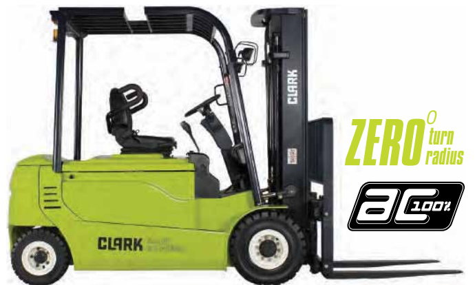
GEX 20/25/30/30s/30L 4-RAD 80 VOLT Elektro-Stapler 20 25 30s 30 30L 2000 2500 3000 3000 3000 KG
